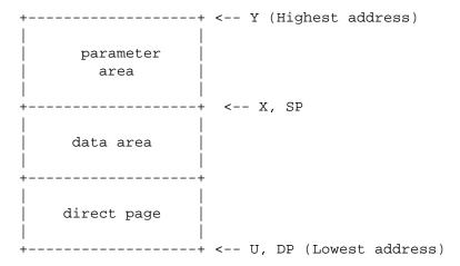
When the process is executed by OS-9, the MPU registers will contain the bounds of the data area: U will contain the beginning address, and Y will contain the ending address. The SP register is set to the ending address+l, unless parameters are used. The direct page register will be set to the page number of the beginning page. If there are no parameters, Y, X, and SP will be the same. Shell will always pass at least an end of line character in the parameter area.
