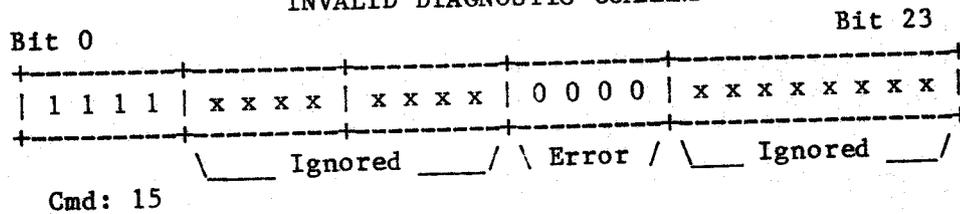
INVALID DIAGNOSTIC COMMAND (Command 15, Function 0) -- The Command Error bit is set and the controller immediately presents ending status. No I/O requests are issued to the Marksman. The diagnostic status byte is set to "F0" (Hex). This command is used to test the command decode and error detection code in the CDS controller.
