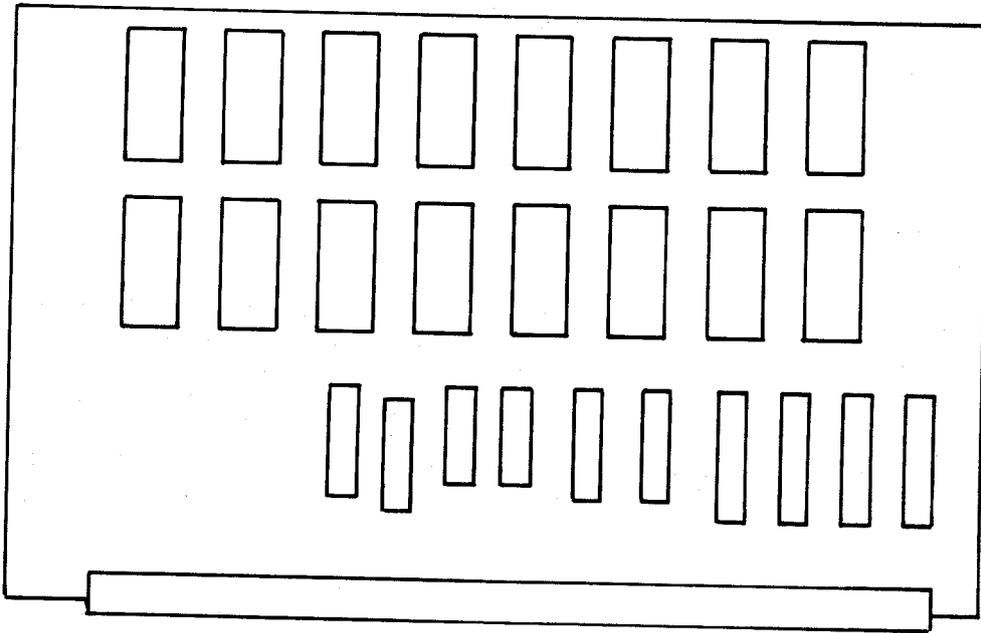
The S-32 Memory board uses CMOS 2K x 8 Static RAMS like Hitachi 6116's. Since each memory chip contains all eight bits of a data word, the bits-in-error field cannot help locate the faulty part. The RAM's on the board are arranged in pairs, to make 4K pages. Note that static RAM's cannot have refresh problems. The RAM chips are in ascending address order, from the top right hand corner proceeding left and down. See the documentation on the S-32 board.
