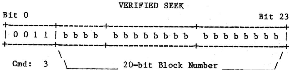
VERIFIED SEEK (Command 3) -- A seek command causes the head mechanism to be positioned over the proper cylinder and the correct head and sector to be selected. The diagnostic status byte is set to "30" (Hex). The 20-bit logical block number is based at zero, and represents the number of the block that will subsequently be processed. The media is mapped to appear as contiguous blocks, with numbers zero to the maximum allowed. The following steps are followed during seek processing:
