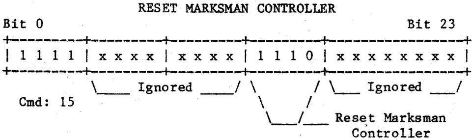
RESET MARKSMAN CONTROLLER (Command 15, Function 15) -- The reset Marksman command sends a drive reset to the Marksman controller. The seek incomplete bit is then set in the primary status byte. If the drive is spinning and ready, this command will cause the front panel "Select" light to momentarily go out. The diagnostic status byte is set to "FF" (Hex).
