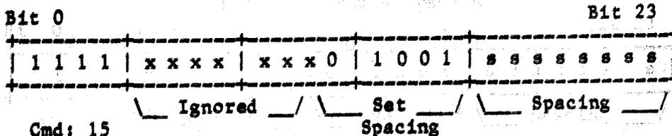
SET DATA SECTOR SPACING (Command 15, Function 9) -- The set data spacing command is used to set the sector interleave used by the CDS controller. This spacing overrides the spacing definition found in the configuration block. Note that this value is not stored in the configuration block on disk, hence it does not permanently change the sector spacing used by the drive. This command is normally used in certain backup procedures. The diagnostic status byte is set to "F9" (Hex).
