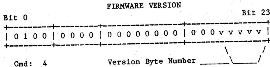
FIRMWARE VERSION (Command 4) -- This command is used to return information regarding the Version Numbers and other information about the SWTPC Controller Firmware. The Version Byte Request Number is used request specific information about the current firmware. The information is returned in the diagnostic status byte. Available information is as follows:
