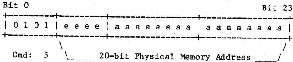
READ BLOCK (Command 5) -- This command reads the selected sector from disk and performs a DMA transfer operation to move the sector to the designated area of memory. The address specified must be a full 20-bit physical address, and the sector buffer must not cross a 4K segment boundary. The diagnostic status byte is set to "50" (Hex). The following steps are followed during read processing:
