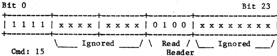
READ SECTOR HEADER (Command 15, Function 4) -- The read header command causes the CDS controller to read the next sector header on the currently selected track. This causes the controller to become oriented with respect to the current track. This command is used to perform seek verification during drive checkout. The diagnostic status byte is set to "F4" (Hex).
