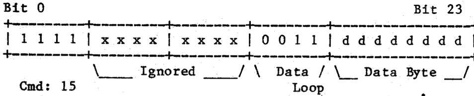
DATA LOOPBACK TEST (Command 15, Function 3) -- The data byte presented by the command is returned to the computer as the diagnostic status byte. This command is normally used to check the integrity of the letterbox data path, including the CDS to Computer cable assembly.
