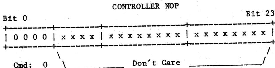
Controller NOP (Command 0) -- The controller immediately presents ending status. Command Error and No Record Found status are reset. The diagnostic status byte is set to "00" (Hex).
