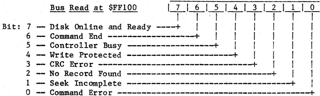
**Disk Online and Ready** -- The MARKSMAN disk unit has been sequenced up and has presented READY status to the controller. This indicates that the drive is up to speed, the controller has been configured (or has determined that it cannot be configured), and no write unsafe condition exists. It is not a write unsafe condition if the media is write protected.
