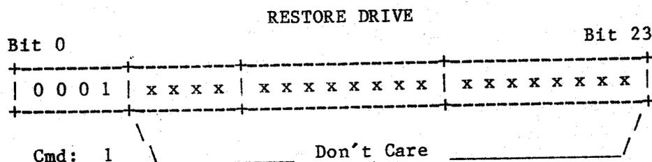
RESTORE DRIVE (Command 1) -- The controller sets the Seek Incomplete status bit, then checks the state of the drive ready bit. If the drive is not ready, Command Error is set and the restore command terminates. Otherwise, a rezero command is issued to the Marksman controller and the track orientation is marked as invalid. The diagnostic status byte is set to "01" (Hex).
