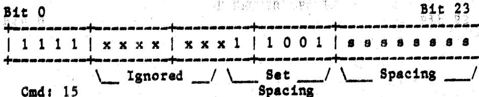
SET SWAP SECTOR SPACING (Command 15, Function 9) -- The set swap spacing command is used to set the sector interleave used by the CDS controller. This spacing overrides the spacing definition found in the configuration block. Note that this value is not stored in the configuration block on disk, hence it does not permanently change the sector spacing used by the drive. The diagnostic status byte is set to "F9" (Hex).
