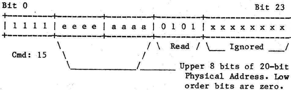
DIAGNOSTIC READ (Command 15, Function 5) -- The diagnostic read command is used to test for soft read errors, and to recover data from sectors that may have CRC errors. For details about read processing, see the documentation on READ BLOCK. Note that normal block retry procedures are suspended by a diagnostic read. The diagnostic status byte is set to "F5" (Hex).
