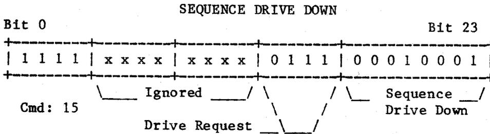
SEQUENCE DRIVE DOWN (Command 15, Function 7) -- The sequence down command is used to spin up the Marksman drive, regardless of the state of the front panel SELECT button. A manual sequence flag is set internal to the controller which is required for operation of certain other commands. The diagnostic status byte is set to "F7" (Hex).
