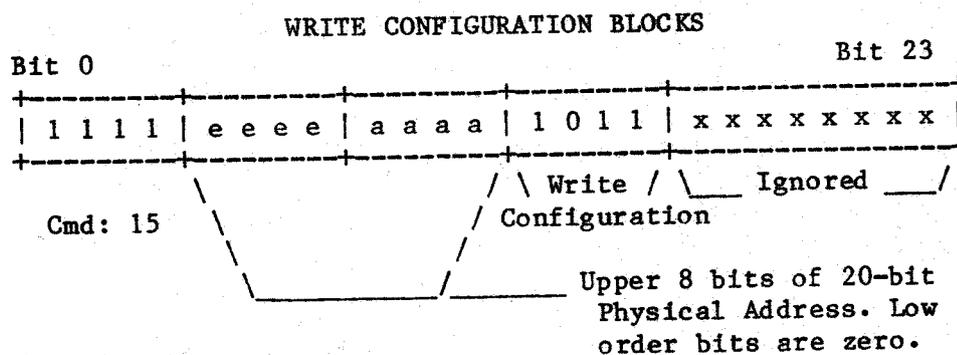
WRITE CONFIGURATION BLOCKS (Command 15, Function 11) -- The write configuration command is used to write the configuration blocks onto the Marksman maintenance track. This track is located on the last head of the last cylinder on the drive. The specified physical address points to the 512-byte configuration block to be written. This block is written into every sector on the last track. If at least one of these blocks is readable, the drive can be configured (See Read Configuration).
