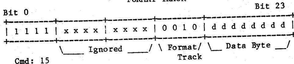
FORMAT TRACK (Command 15, Function 2) -- The format track command is used to write format information on an entire track of the Marksman media. This command performs the same function as the Format Block command, except that an entire track is processed (in 100 mSec.) as opposed to one block (in 25 mSec.). The blocks written on the track are filled with the data byte field. For normal formatting, a data byte of zero is recommended.
