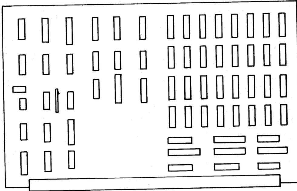
The M-256 memory board uses NMOS 64K x 1 RAMs like MCM6665 or TMS4164's. The parts must have a maximum access time of 200 Nsec and a maximum cycle time of 375 Nsec. Refresh is implemented using an 8-bit row counter and a 1.5 mSec power reduction timer. A refresh cycle is conducted on each bus cycle that is not a board access until the entire array is refreshed. Refresh is then suspended until the 1.5 mSec timer starts a new refresh group. See the M-256 documentation.
