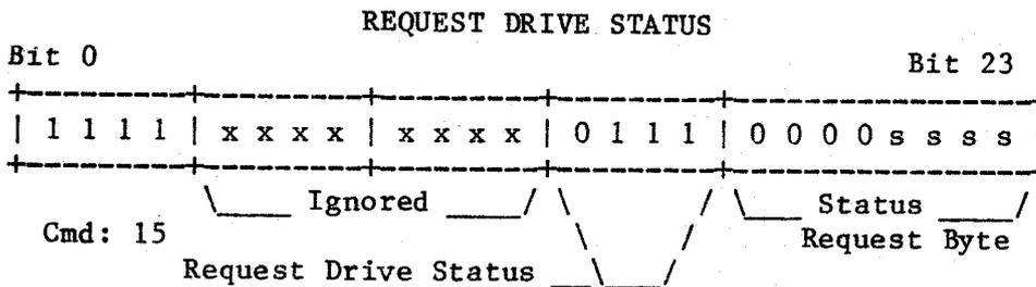
REQUEST DRIVE STATUS (Command 15, Function 7) -- The request status command interrogates the Marksman controller for status. The particular status byte requested is returned as the diagnostic status byte. The meaning of this status byte is documented in the Marksman Performance Specification, Century Data Systems document #76220-906. Note that not all revisions of the Marksman controller have extended status.
