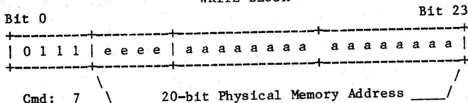
WRITE BLOCK (Command 7) -- This command performs a DMA transfer to obtain the specified buffer from the host computer. The buffer is then written to the selected sector on disk. The address specified must be a full 20-bit physical address, and the sector buffer must not cross a 4K segment boundary. The diagnostic status byte is set to "70" (Hex). The following steps are followed during write processing:
