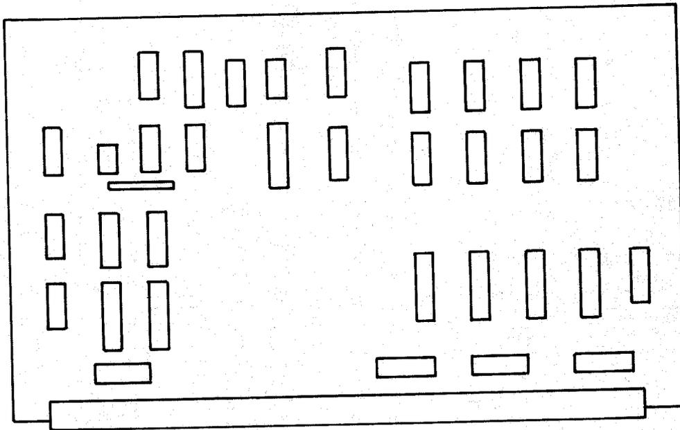
The M-64 Memory board uses NMOS 64K x 1 dynamic RAMs like Hitachi 4864-3's or TMS 4164's. The maximum access time on these RAMs is 200 nSec., with a maximum cycle time of 375 nSec. Refresh is implemented with an 8-bit row counter and a refresh cycle is conducted on every bus cycle that does not access the memory board. A fail-safe timer is used to halt the processor if necessary to guarantee refresh. For bit definitions, see the documentation on the M-64 memory board.
