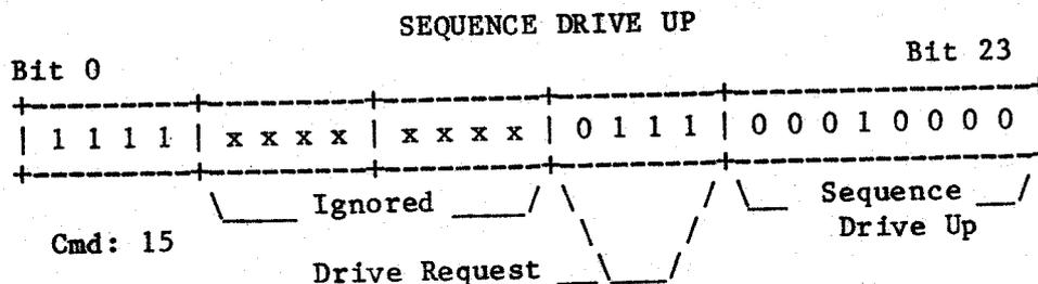
SEQUENCE DRIVE UP (Command 15, Function 7) -- The sequence up command is used to spin up the Marksman drive, regardless of the state of the front panel SELECT button. A manual sequence flag is set internal to the controller which is required for operation of certain other commands. The process of sequencing consists of the following steps:
