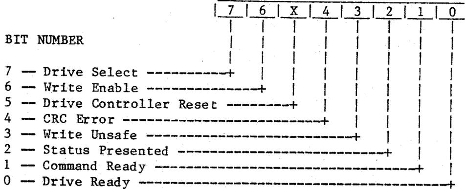
**Drive Select** -- This bit reflects the status of the front panel SELECT button. When high (one), the button indicates that the drive should be sequenced up. Note that this signal does not directly affect the ready or not ready status of the drive.
