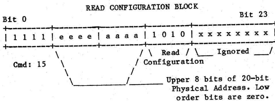
READ CONFIGURATION BLOCK (Command 15, Function 10) -- The Read Configuration command is used to initialize certain control tables from one of the configuration blocks recorded on the last track of the disk. The diagnostic status byte is set to "F5" (Hex).
