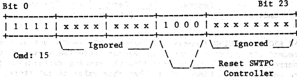
RESET SWTPC CONTROLLER (Command 15, Function 8) -- The Controller Reset command causes a software reset of the CDS controller. A reset indication is presented to the Marksman Controller. An interrupt is returned to the computer upon completion of the reset processing, but no valid status is returned.
